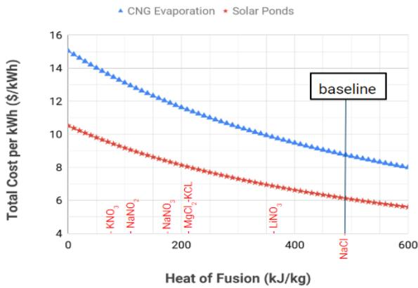
Fig. 9. The effect of ROC salt heat of fusion on the normalized TES cost.
