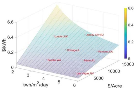
Fig. 6. Normalized TES cost using evaporation ponds in different locations.  $C_{tes}$  is plotted with respect to local cost of land  $C_l$  and solar irradiance,  $I$ .
