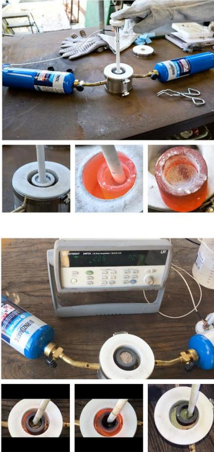
Fig. 2. Verification of solid to liquid phase change on ROC salt content. No phase change observed in the sample from CDA (top). Solid to liquid phase change observed in the sample from EMWD between 350-400 °C (bottom).
