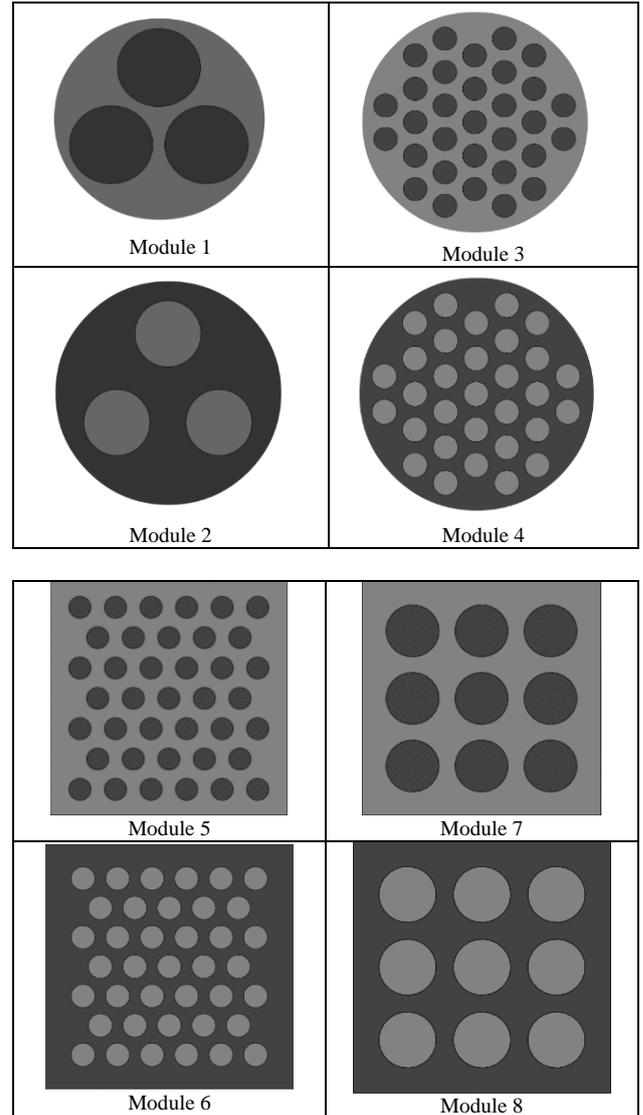
Fig. 3. Different containment designs of the TES module. The volume of ROC salt is equal in all cases. Module 8 corresponds to the minimum overall TES cost (baseline) – Dark color: ROC Salt, light color: heat transfer fluid.
