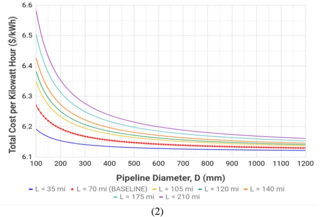
Fig. 4. Effect of the distance between RO and ROC processing facilities and pipeline diameter on the total normalized TES cost using 1- CNG and 2- Solar Pond.
