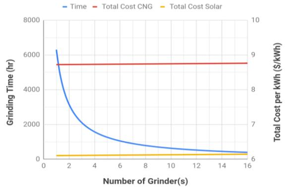
Fig. 7. Effect of the number of commercial grinders on the processing time and the normalized cost of TES using CNG and Solar ponds. Baseline case assumes 3 grinders.
