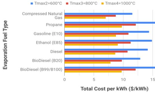
Fig. 5. Sensitivity of normalized cost of ROC-based TES system with respect to evaporation fuel type.
