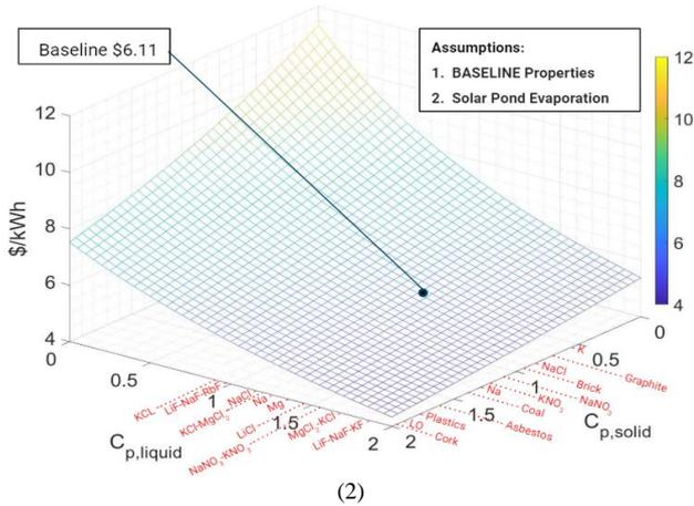
Fig. 8. The effect of heat capacity of the ROC salt in solid and liquid on the normalized TES cost: (1) using CNG to evaporate the; (2) using solar evaporation pond.
