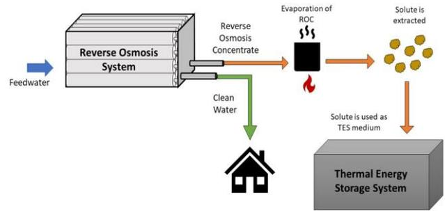
Fig. 1. Development of an ROC-based thermal energy storage system.
