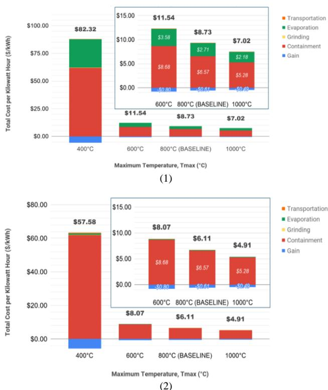
Fig. 12. Summary of sensitivity analysis; comparison of different costs/gain on the normalized TES cost using (1) CNG and (2) solar ponds for evaporation.
