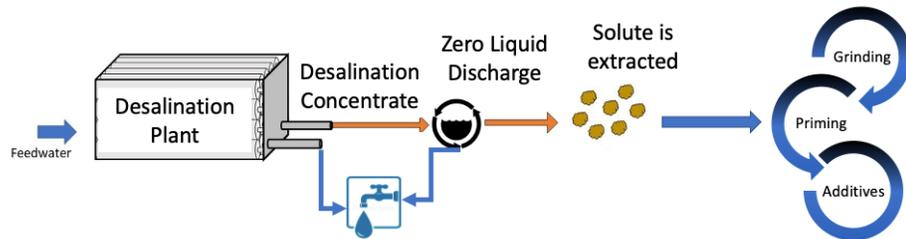
*Figure 1 – Development of a concentrate-based thermal energy storage module*
