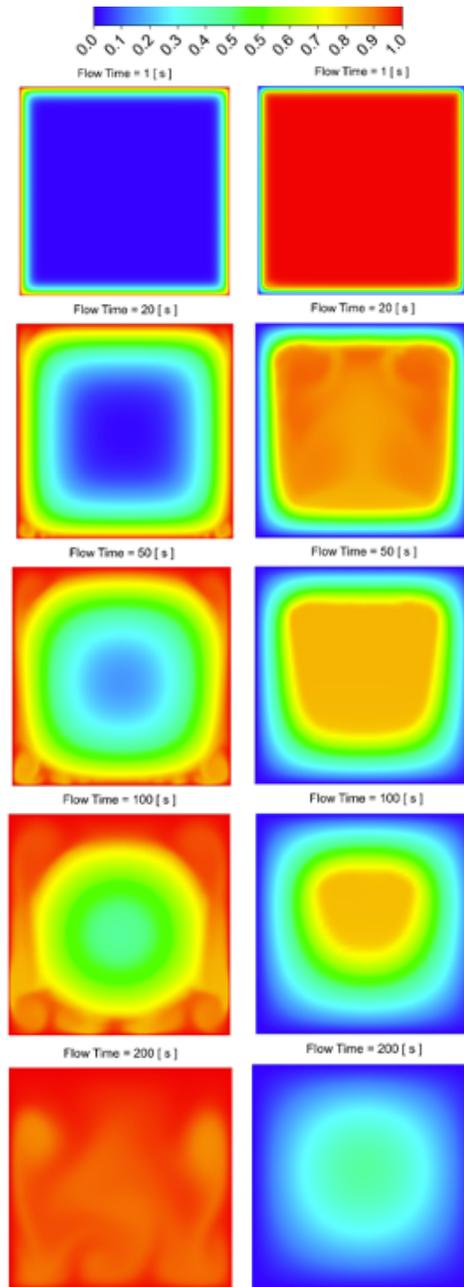
**Figure 3 – Time-lapse of charge (left) and discharge (right) showing contour plots of dimensionless temperature**
