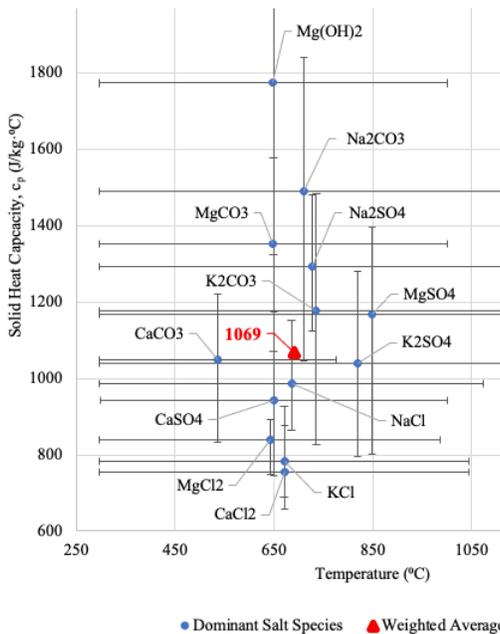
**Figure 2 – Heat capacity of dominant salt species in desalination salt**
