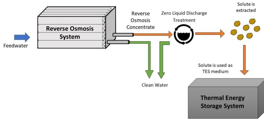
Figure 9: Development of ROC-based TES System
