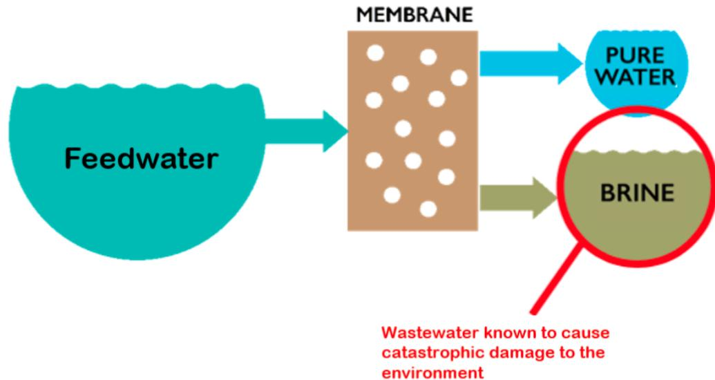
*Figure 2: Membrane Process for Desalination*
