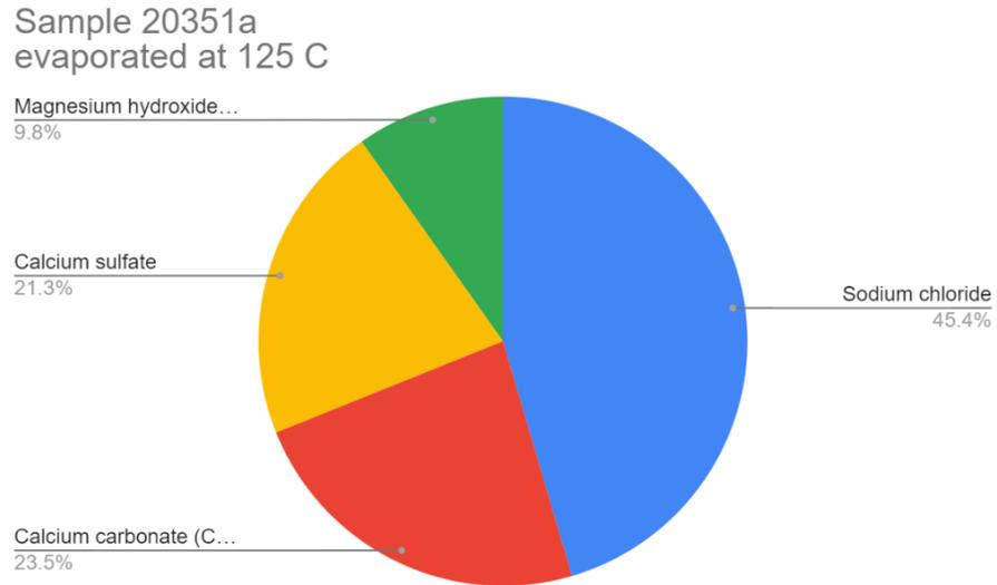
*Figure 17: Chemical Composition of EMWD ROC Sample*
