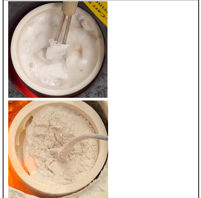
Figure 2 – Right: The ROC salt from Panoche Water District at 400 °C – Left: The molten ROC salt sample at 600 °C
