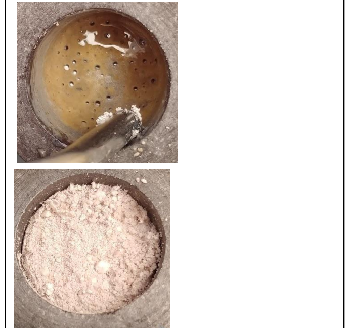
Figure 2 – Right: The ROC salt from Panoche Water District at 400 °C – Left: The molten ROC salt sample at 600 °C
